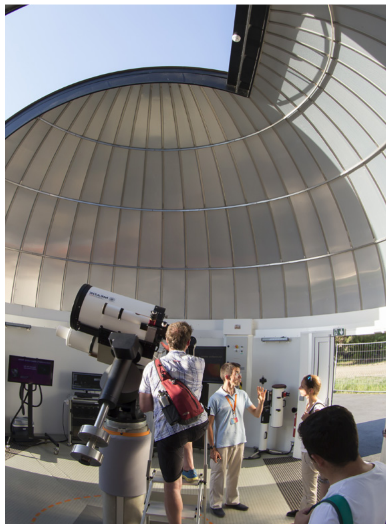
Under its 7.5m-diameter dome, a 40-centimetre telescope and a telescope dedicated to observing the Sun are housed.
